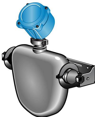
Figure 2-11: CMFS025, CMFS040, or CMFS050 wall mounted using bracket
